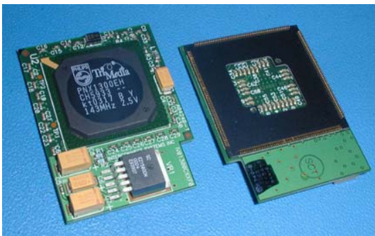
BGA to QFP Adapter with VR using FlexFrame™ Interconnect
